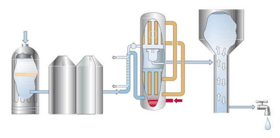
Distillation is being explained in the following via individual subprocesses.
